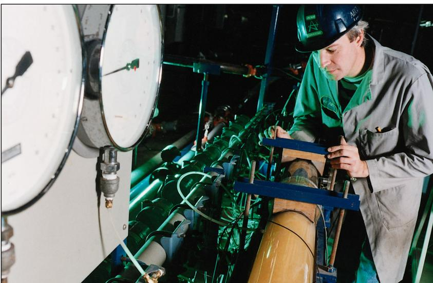
*A flow visualization test is conducted at AECL's Sheridan Park Engineering Laboratory. Such tests ensure a clear understanding of fuel behaviour in the reactor. Meeting stringent safety criteria is the first priority of all AECL systems.*
