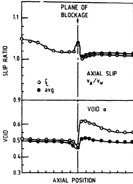
Fig. 6. Computed void fraction and slip ratio, average and centre line values (peripheral).
