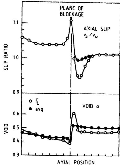
Fig. 7. Computed void fraction and slip ratio, average and centre line values (central).
