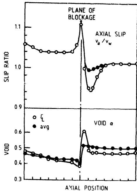
Fig. 7. Computed void fraction and slip ratio, average and centre line values (central).
