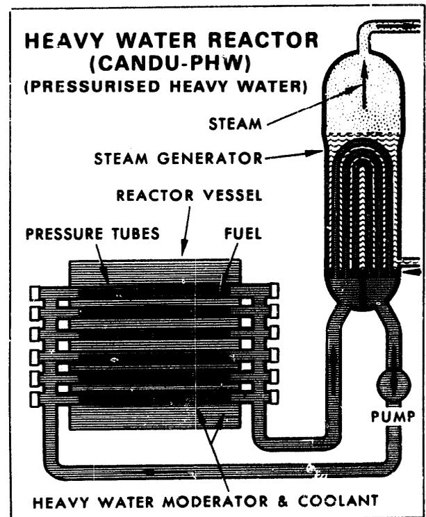
Fig. 1. Simplified view of CANDU reactor showing flow paths.
