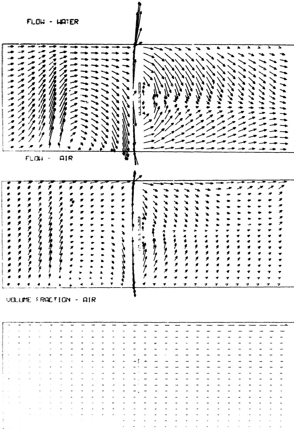
Fig. 5. Computed volumetric flow fields and void fraction profile for the central blockage.
