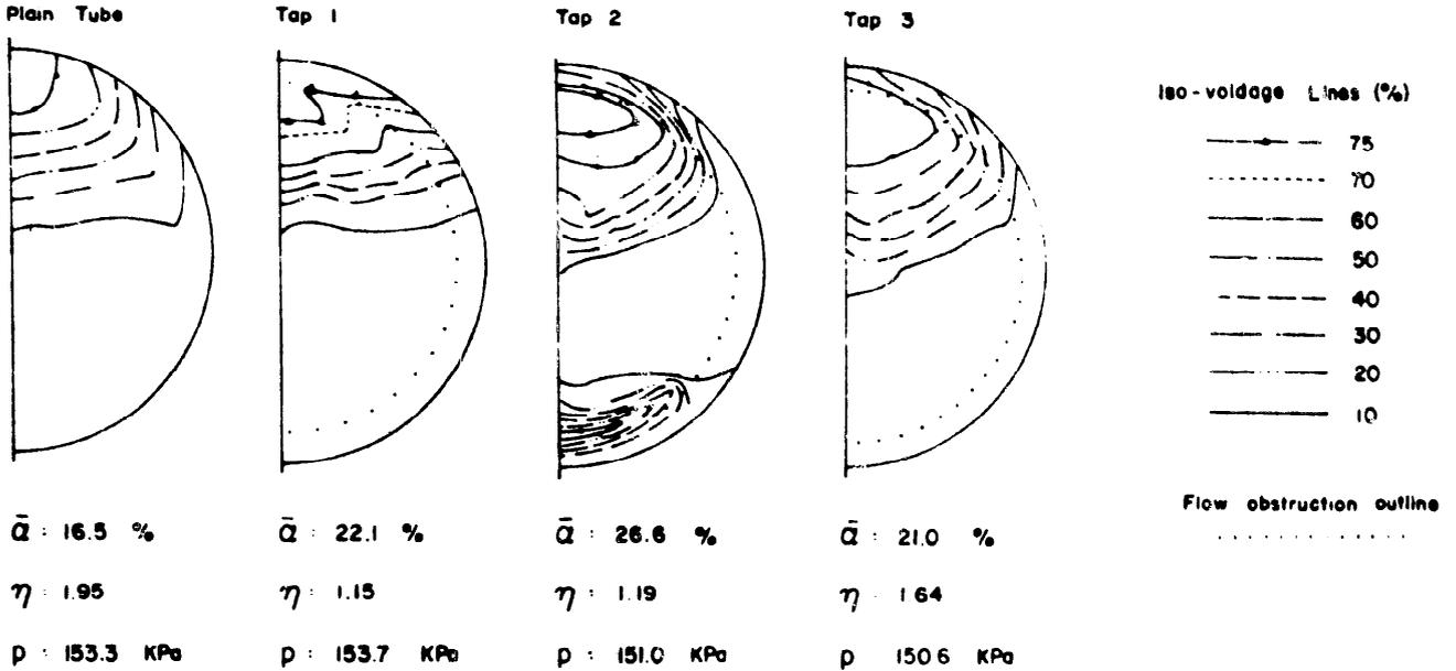
(a). Change of void distribution. Peripheral obstruction. Bubbly flow. Water: 1.1 kg/s. Air: 0.000775 kg/s. Quality: 0.0704%.
