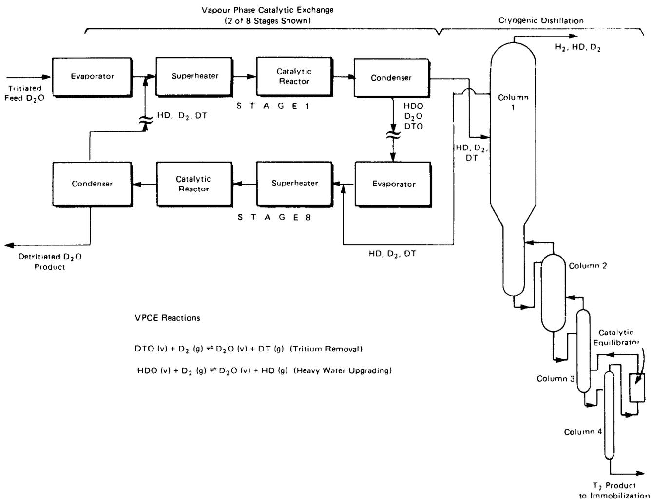
Figure 1: Darlington Tritium Removal Facility process flow diagram.
