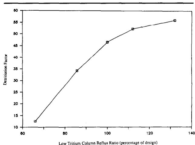
**Figure 4:** The effect of varying the reflux ratio in the first column (Low Tritium Column) in the cryogenic distillation cascade.
