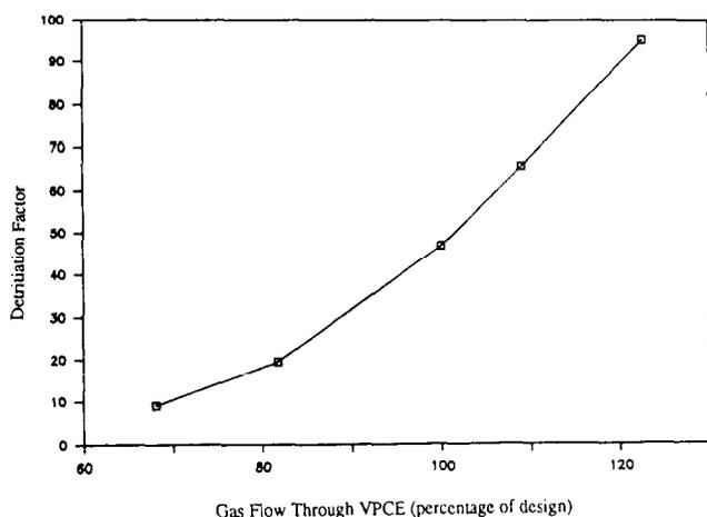
**Figure 3:** Relationship between detritiation factor and deuterium gas flow through the VPCE. The reflux ratio in the first column of the cryogenic distillation (the Low Tritium Column) is assumed to be held constant.
