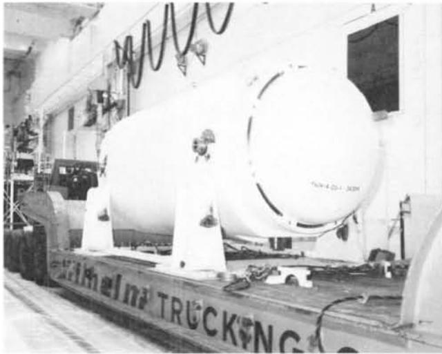
**Figure 3:** The second storage cask (TN-24P) built by Transnuclear, Inc.
