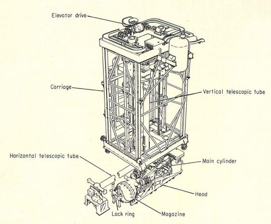
REFUELING-MACHINE HEAD has pneumatically operated lock ring that seals onto fuel-channel end fitting. After the two machines (one loaded with five new fuel bundles, the other empty and ready to take five spent-fuel bundles) are clamped onto opposite ends of a fuel channel, heads are filled with D<sub>2</sub>O and pressurized to match reactor pressure, machines remove end-closure plugs from channel and store them in magazines within heads. Then
