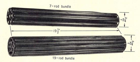
FUEL BUNDLES, which are of two types, all contain natural-UO<sub>2</sub> pellets in Zircaloy-2 tubes that are spaced by Zircaloy wires wrapped and spotwelded around tubes in double-course helix. Wires also cause coolant mixing; nine fuel bundles are loaded
