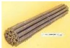
**Description:** The design has now matured and the split-spacers are now canted to prevent interlocking and a full length bearing pad has been added in the center plane. This bundle has seen endurance testing in the Sheridan Park loop and the braze alloy has a higher corrosion rate than the normal Zircaloy, thus the white appearance at the joints of the bearing pads.
