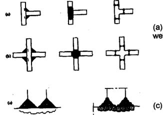
(a) & (b) replace fillets with solid weld metal or forgings
