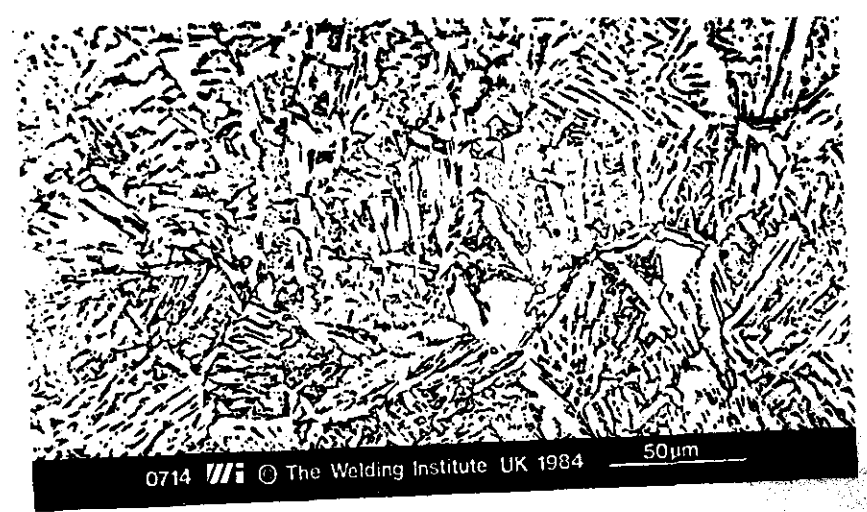
A view at higher magnification of part of the heat affected zone shown in slide 0712, towards the fusion boundary, but farther from it than slide 0713, heated to a temperature above A_{c3} , but insufficient to produce rapid austenite grain growth.
