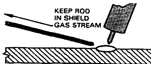
Withdraw Rod Slightly from the Weld Pool
