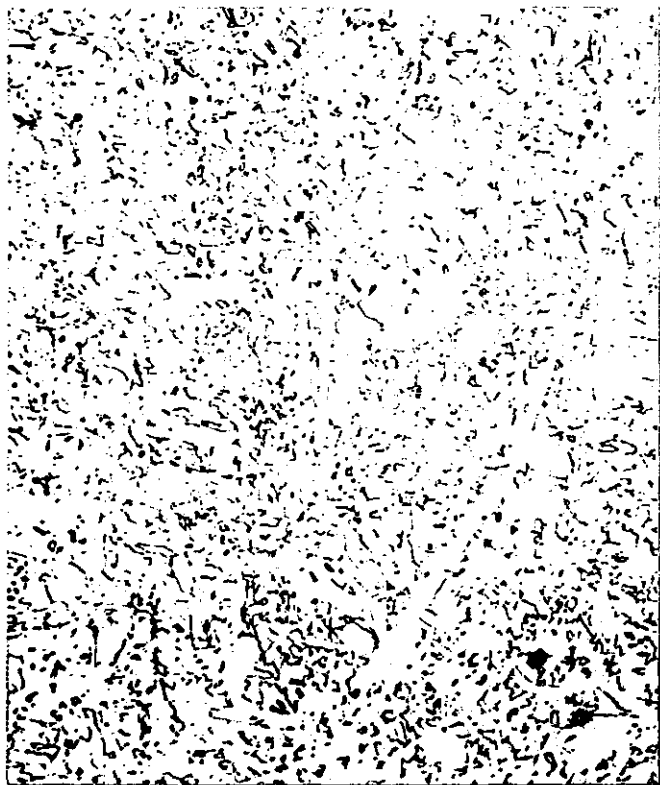
Fig. 8 — Microstructure of weld metal deposited by ESW at 25 kJ/mm using EWT-G filler metal. 400X.
