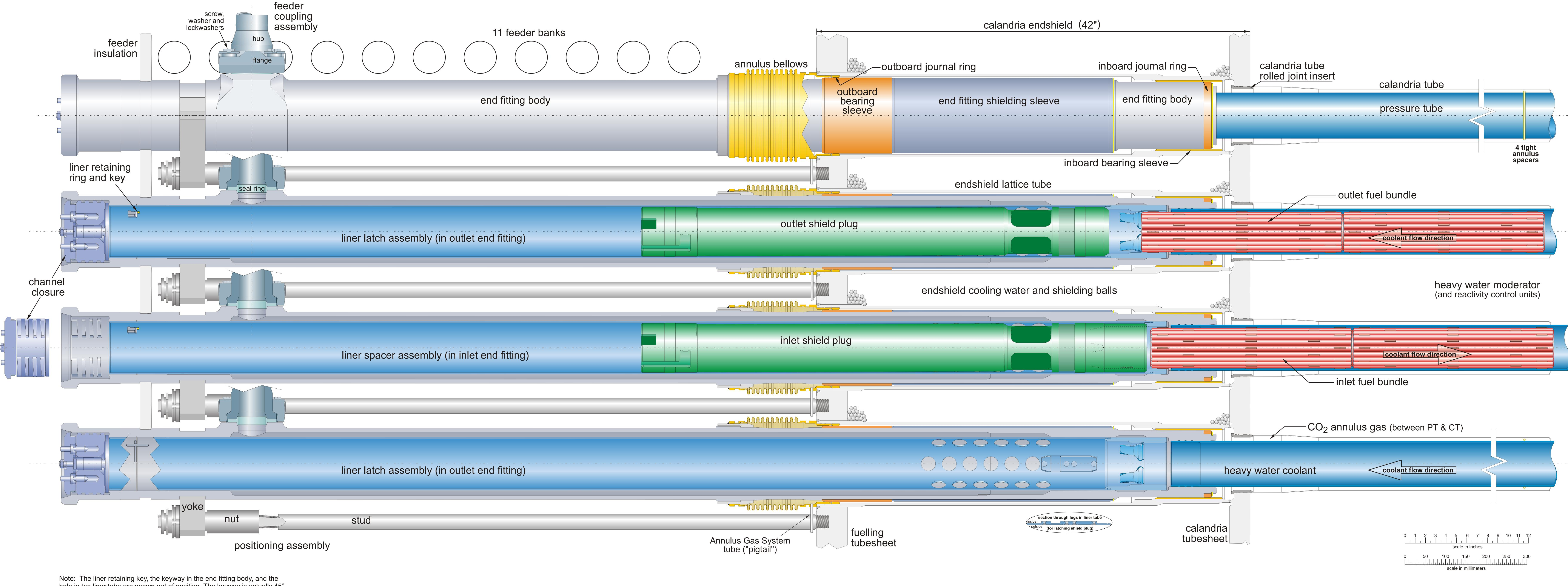
Note: The liner retaining key, the keyway in the end fitting body, and the hole in the liner tube are shown out of position. The keyway is actually 45° to the right of top centre, when looking into the end of the end fitting. Similarly, feeder couplings are generally above center and positioning assemblies below center. The positioning assemblies are oriented to avoid obstructing the feeder couplings.
