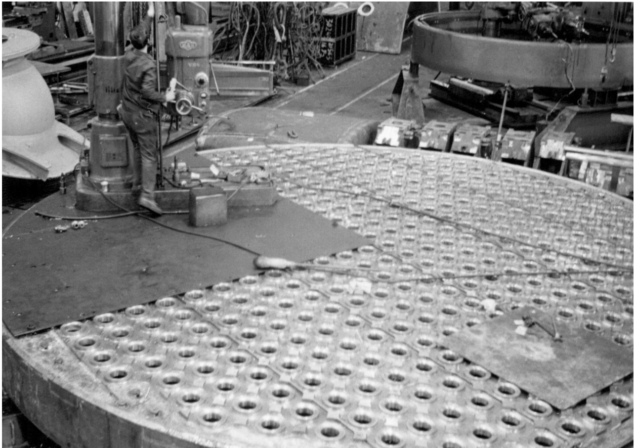
Figure 3 Milling the inside face of the calandria tubesheet
