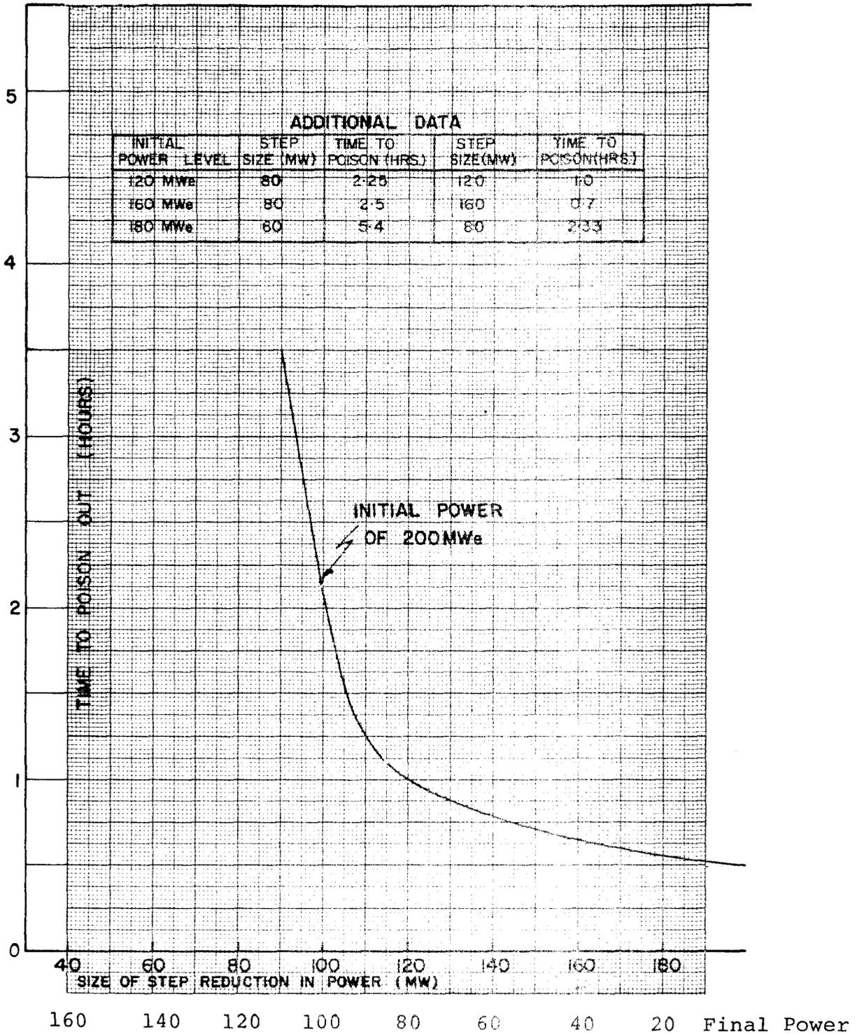
Time to Poison Versus Size of Step Reduction in Power from an Initial Power Level of 200 MWe. Values for Other Initial Power Levels are Shown in Tabular Form. Fuel Assumed to be at Equilibrium Irradiation.
