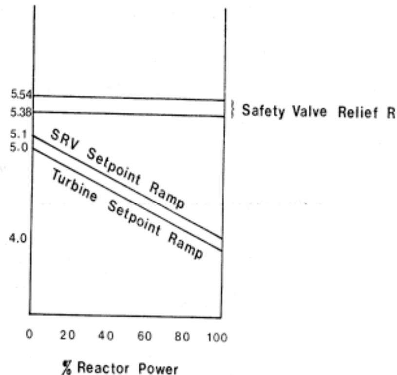
Figure 5: Steam Pressure Operating Diagram.
