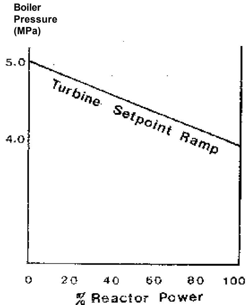
Figure 2: Ramped Boiler Pressure.
