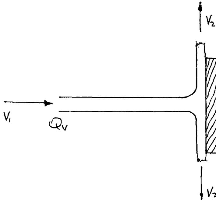
Consider a jet striking a flat plate. The final velocity of the fluid is at  $90^\circ$  to the original velocity and the jet is split in radial directions, thus  $V_2$  is zero. Thus the change in velocity =  $V_2 - V_1 = 0 - V_1$ . Thus the force exerted by the plate, to deflect the jet, has to act in the opposite direction to the flow.
