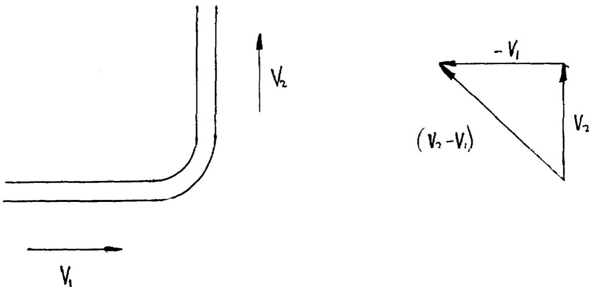
The change in velocity =  $V_2 - V_1$ . ( $V_2 - V_1$ ) is the direction in which the force has to be applied to prevent the pipework moving.
