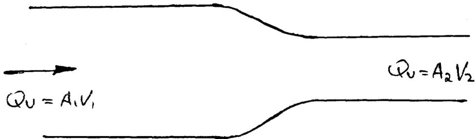
$$\text{Force on nozzle} = \ell \times Q_v \times (V_2 - V_1)$$
