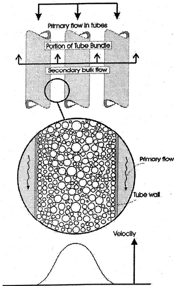
Figure 1. Tube-Coolant Interface
