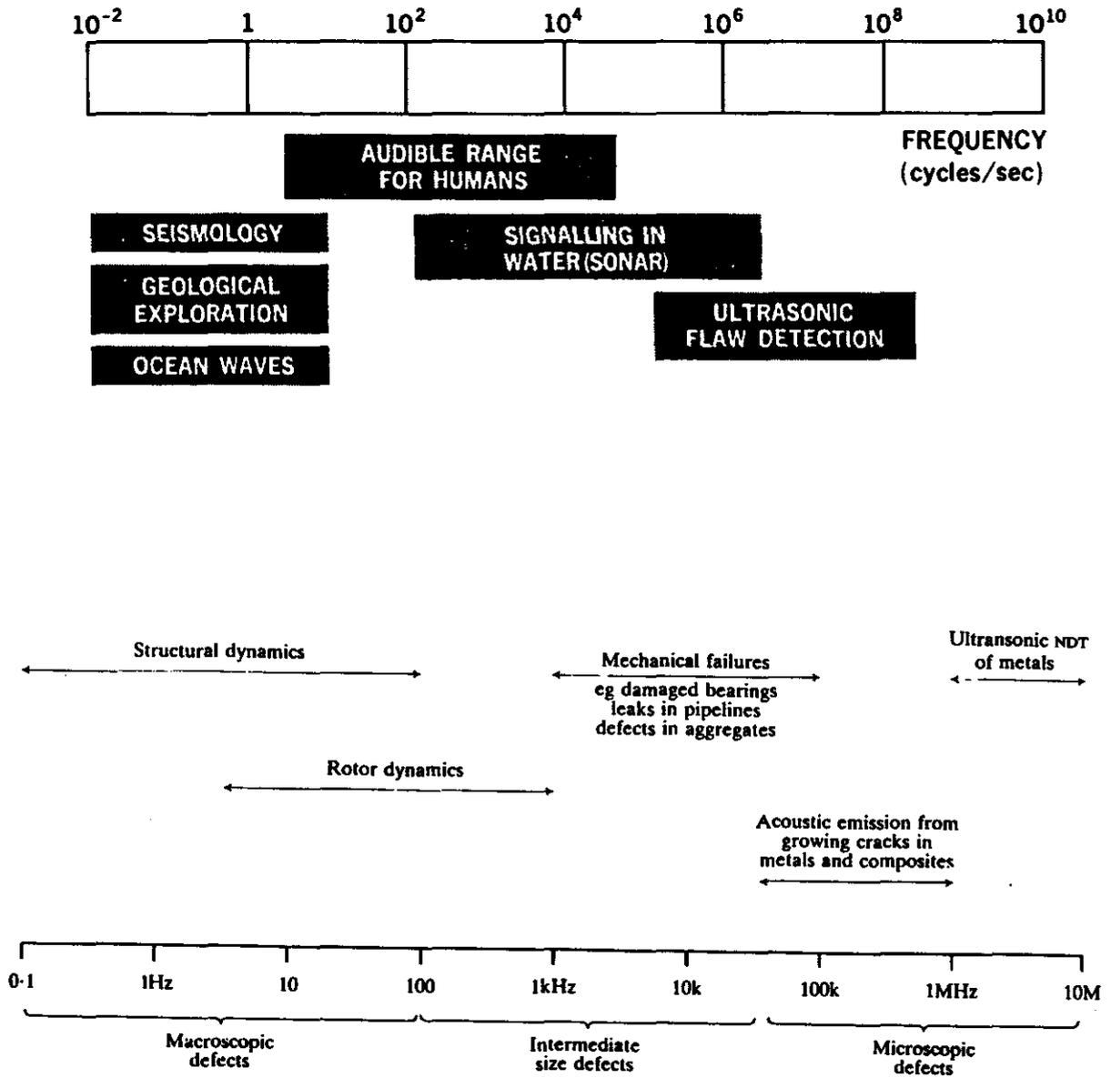
Figure 1.2: Mechanical Vibrations and Sound Spectrum
