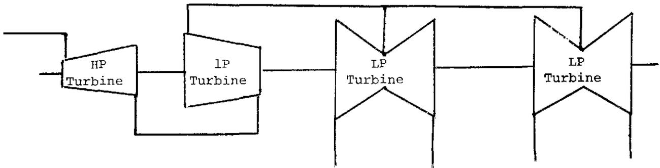
The diagram above is of a four casing turbine unit used at a conventionally fired, superheated steam generating station. Discuss possible reasons for:
