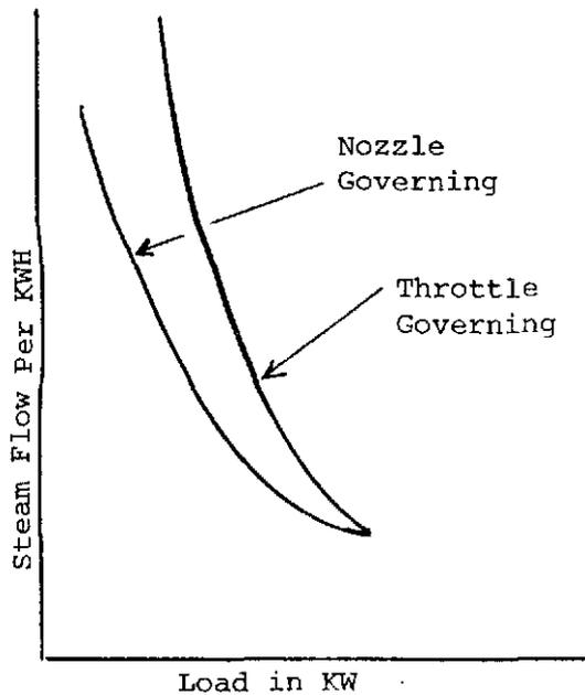
Figure 1.22 is a comparison of steam rates for nozzle and throttle governing. The nozzle governed turbine consumes less steam per kilowatt-hour for all power levels up to the maximum. The nozzle governed turbine is more efficient as a variable load turbine; however, a base load turbine which seldom runs below full power can obtain good efficiency with a much simpler governing system.
