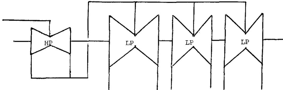
The diagram above is of a four casing turbine unit used at a nuclear fuel, saturated steam generating station. Discuss possible reasons for:
