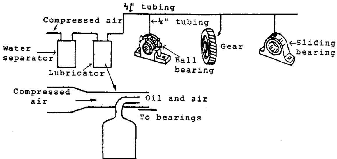
LUBRICATING AEROSOL carries fine oil particles in suspension until they hit moving surface. Shaft movement drags oil from airborne mixture into the bearing surfaces.
