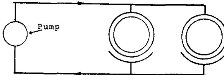
EXTERNAL PUMP assures constant oil supply. After passing through bearings, the oil is collected and recirculated, reducing consumption
