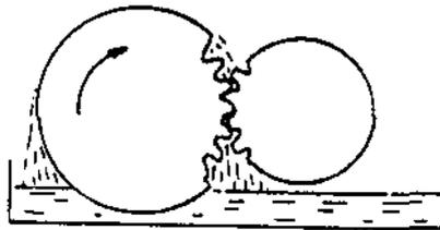
SPLASH LUBRICATION is simple form of circulating system (like a ring oiler). Oil is carried to pressure area by clinging on the teeth
