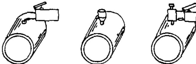
GREASE FED to bearing by spring pressure from reservoir, right. Spring compresses each time unit is filled from outside grease gun
