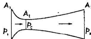
In the convergent section of a nozzle, the initial flow is subsonic and the velocity is accelerated as the gas approaches the throat which is the area of minimum cross section. The maximum velocity at the throat occurs when there is sonic velocity
