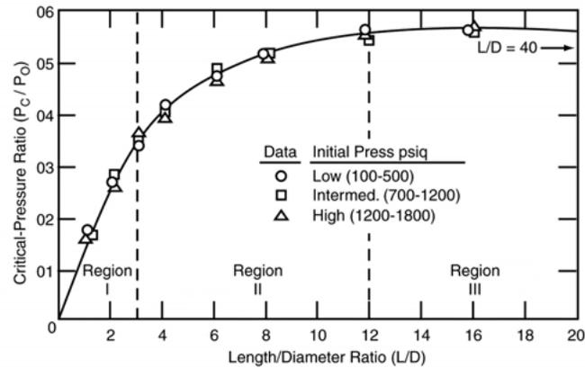
EXPERIMENTAL CRITICAL PRESSURE RATIO DATA AS A FUNCTION OF LENGTH/DIAMETER RATIO
