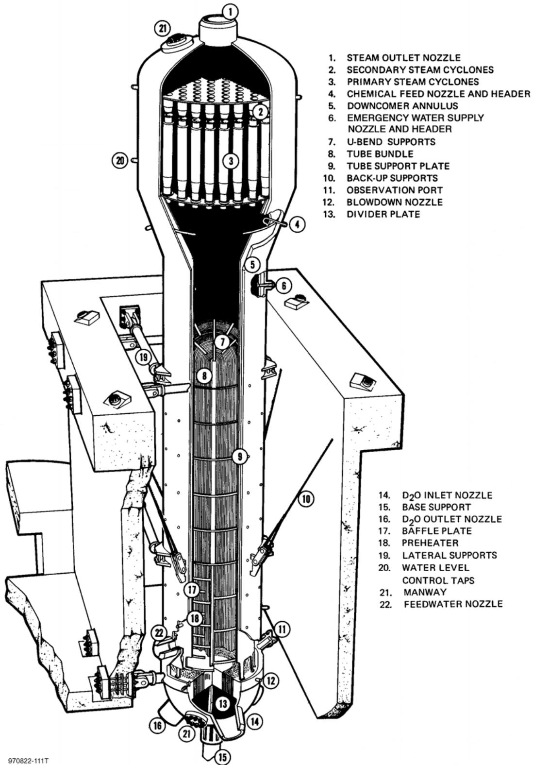
FIGURE 8.6 STEAM GENERATOR FOR 600 MW(e) N.P.S.
