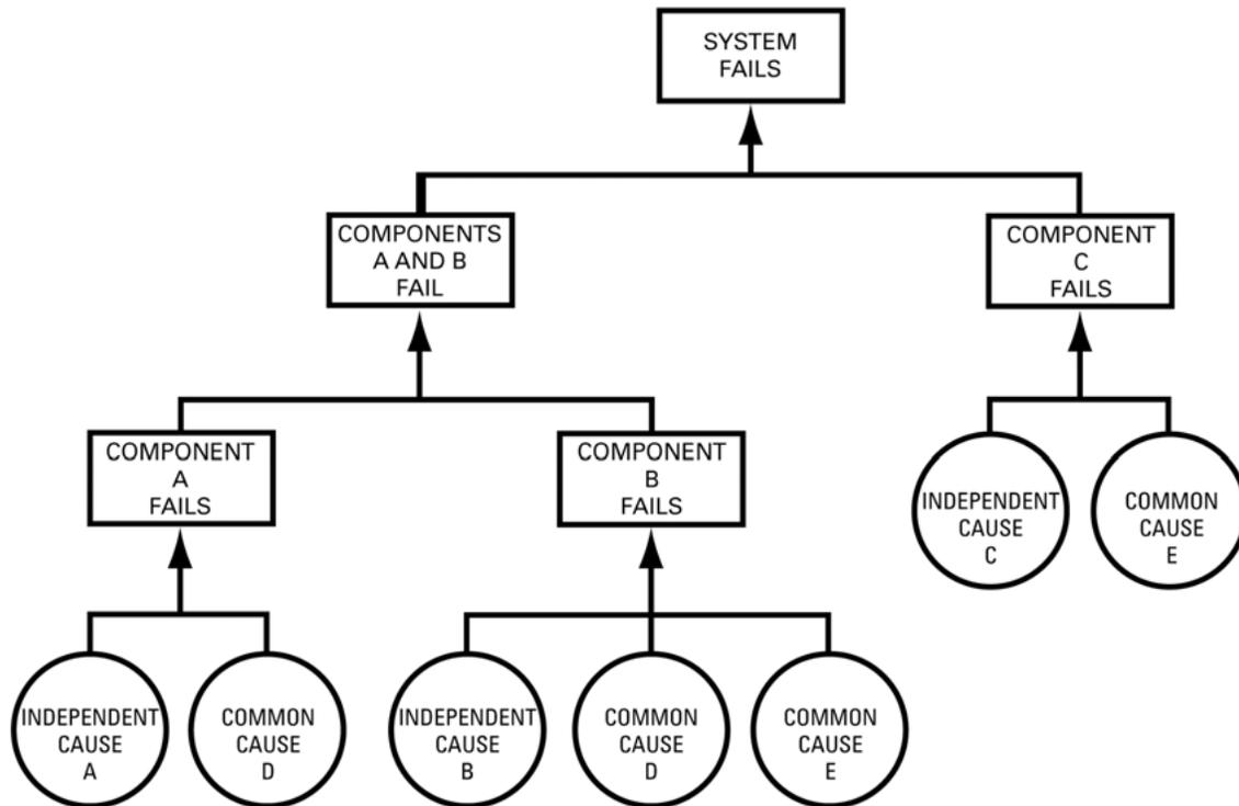
**FIGURE 5.6 – COMMON - CAUSE FAILURE ANALYSIS**
