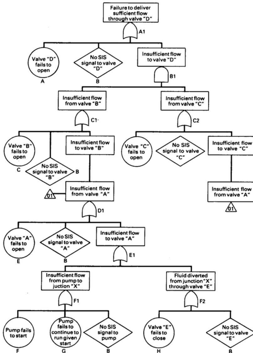
Figure 5.2 -- "Failure to Inject" fault tree, labelled for Boolean reduction
