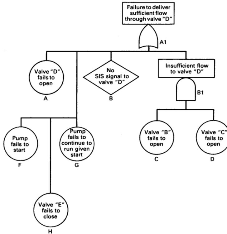
Figure 5.4 -- Injection system mincut fault tree equivalent to fault tree shown in Figure 5.2
