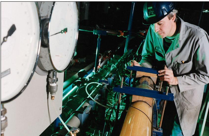
A flow visualization test is conducted at AECL's Sheridan Park Engineering Laboratory. Such tests ensure a clear understanding of fuel behaviour in the reactor. Meeting stringent safety criteria is the first priority of all AECL systems.
