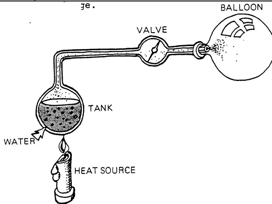
**Figure 1 Steam-boiler experiment**
